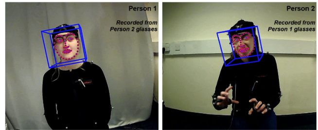
Figure 1: Dyad recording setup. Person 1 and 2 are seated in front of each other. The footage is recording from a camera on each person's PupilLab Glasses. The blue box and the facial landmarks are exported from OpenFace software and added to the original video.
